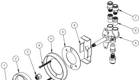
ITEM #9 INCLUDES: DIVERTER VALVE BODY & (2) PHILLIPS HEAD LONG SCREWS
