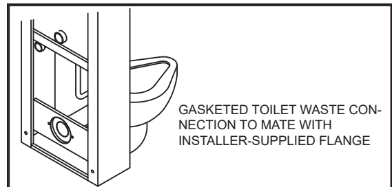
(GWC)- GASKETED WASTE CONNECTION (WALL OUTLET SHOWN)
