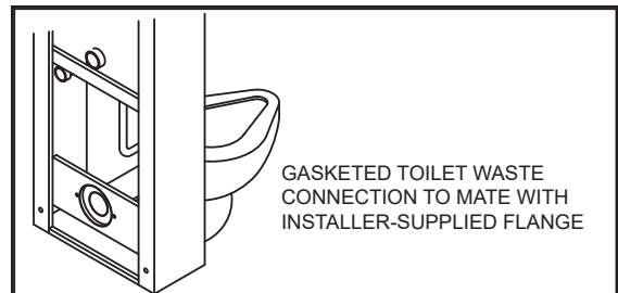
(GWC)- GASKETED WASTE CONNECTION (WALL OUTLET SHOWN)
