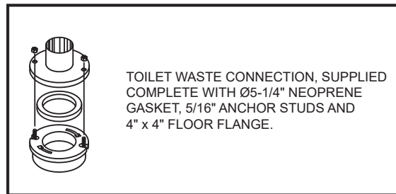
(TW4) FLOOR OUTLET WASTE CONNECTION
