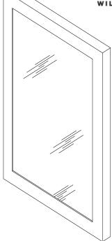
**FMR1** framed security mirror to be 16 GA, Type 304 stainless steel, polished to a #8 non-directional mirror finish. Mirror shall be reinforced with 1/2" fiberboard backing. Anchoring shall be by a 6-point system: threaded rods, nuts and washers furnished for walls up to 8" thick. Unit requires chase for installation.
