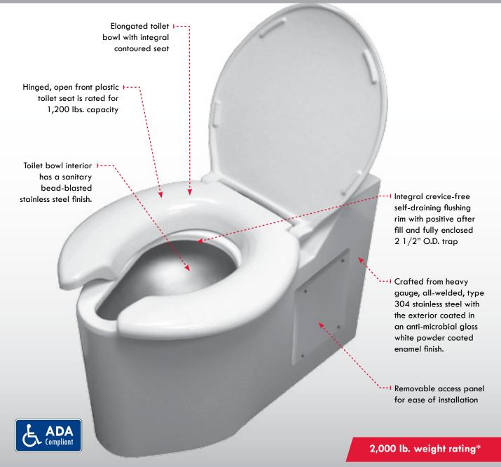
\* The fixture (less hinged seat) will withstand loadings up to 2,000 pounds with no measurable deflection and loadings up to 5,000 pounds with no permanent damage. Bariatric toilet seat is rated for 1,200 pounds. Anti-microbial gloss white powder coating does not protect users against bacteria, viruses, or other disease organisms. Always use good hygienic cleaning practices.
